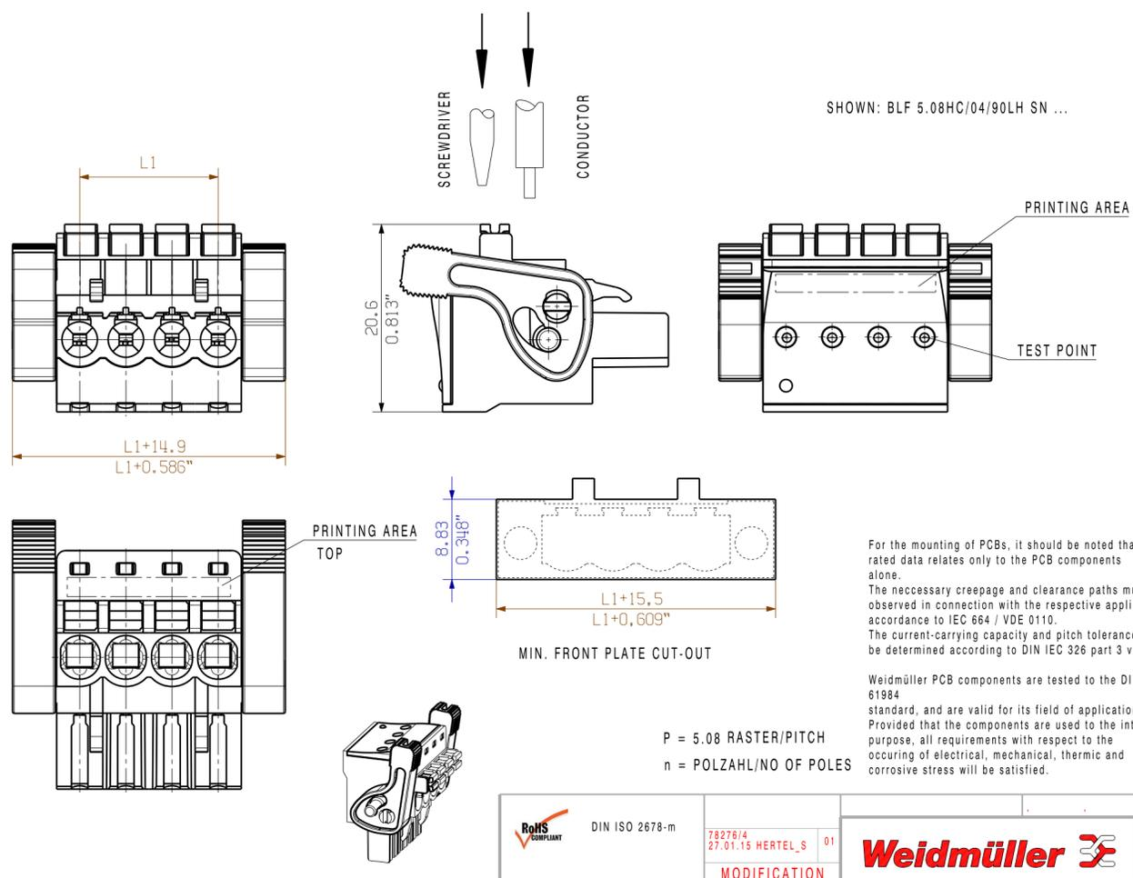
For the mounting of PCBs, it should be noted that the rated data relates only to the PCB components alone. The necessary creepage and clearance paths must be observed in connection with the respective applicant in accordance to IEC 664 / VDE 0110. The current-carrying capacity and pitch tolerance is to be determined according to DIN IEC 326 part 3 very fine.
