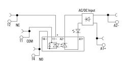
\*Contact is assembled in socket but not used with solid-state relays
