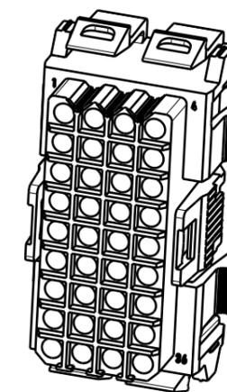
For the mounting of PCBs, it should be noted that the rated data given in the catalogue relates only to the connection elements. The necessary creepage and clearance paths must be observed in connection with the respective applicant in accordance to VDE 0110. The current-carrying capacity and pitch tolerance is to be determined according to DIN IEC 326 part 3 very fine.
