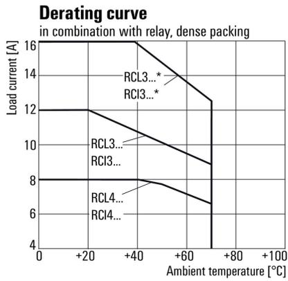
\* For full continuous current (16 A), the wire terminals 11 with 21, 12 with 22 and 14 with 24 must be bridged with a wire  $\geq 1,5 \text{ mm}^2$  at the socket.
