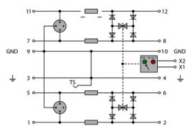
Complete module direct grounding, with remote signalling
