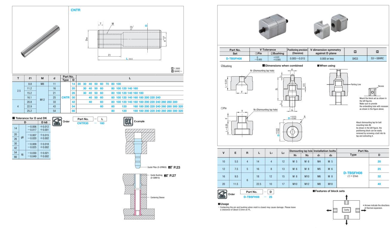
· The block sets are capable of offsetting the plate's thermal expansion caused in high temperature molding process for thermosetting resins, etc., thereby maintaining positioning accuracy. The pin type positioning method cannot thoroughly absorb thermal expansion when it takes place in directions as shown in the figure above. The block type will be unaffected if the groove direction is in parallel to the
