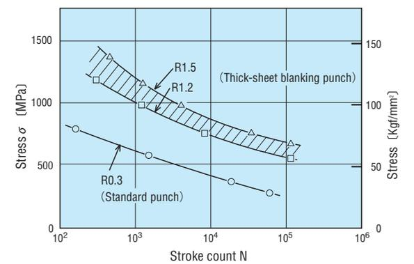
[Fig. 7] Fatigue strength of thick-sheet punch and standard punch (D=5, M2)
