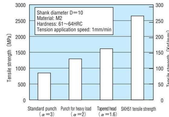
[Fig. 6] Punch head tensile strengths for different punches (D=10, M2)
