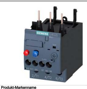
UEBERLASTRELAIS 14...20 A FUER MOTORSCHUTZ BGR S0, CLASS 10, SCHUETZANBAU HAUPTSTROMKR.: SCHRAUBANS. HILFSSTROMKR.: SCHRAUBANS. HAND-AUTOMATIK-RESET
