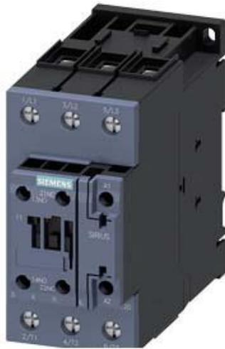
SCHUETZ,AC3:30KW/400V, 1S+1OE, AC/DC 20-33V, M.
