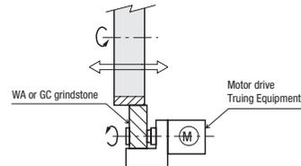
This equipment uses motor drive to rotate the WA or GC grindstone, truing and dressing the wheel. It produces the stablest wheel surface, fast work, and safety.
