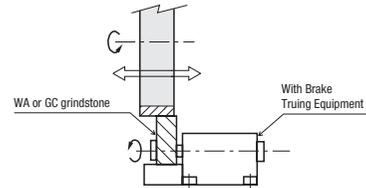
As in the figure, this equipment uses the rotation force of the wheel to rotate the WA or GC grindstone, carrying out truing and dressing through the speed difference between the wheel and the grindstone. Efficient work is possible, but take care as if the grindstone is not properly rotated it may damage the machine.
