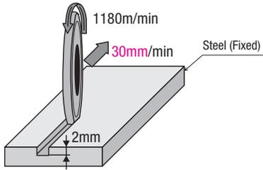
Mark the wheel outer surface with a magic marker etc., and grind raw material such as S45C normally until the entire surface is in contact (the mark is concealed) and there is no more center runout. Dressing is completed along with truing, allowing the actual work to begin.
