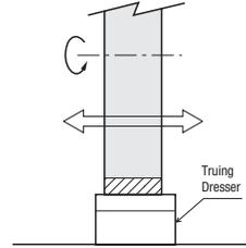
Carry out truing (reflection removing, molding) with the dresser as in the above figure. Wheel sharpness suffers when the truing dresser is used, meaning dressing is required. Take care, however, as cutting beyond reasonable limits will lead to damage to the wheel.
